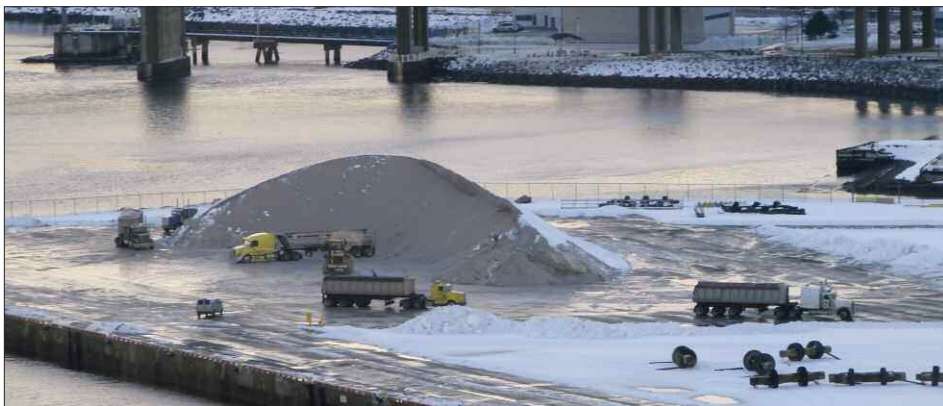
Trucks are loaded with limestone which improves air quality from power plant emissions.
